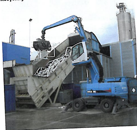
Used window frames are loaded on to a conveyor for shredding
